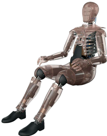
Figure 4: A crash test dummy is an example of an instrumented physical model
